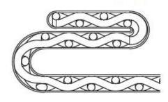
Side Tensioned Bent Hooks Only (E).
